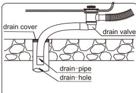
Insert the drain-pipe to the drain-hole on the floor, and then cover it with water retaining cover to prevent waste water spilling.
