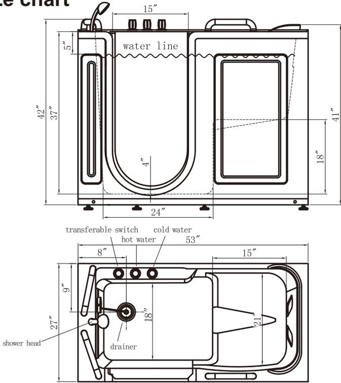
● Water and electricity installation drawing
