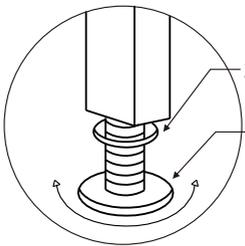
2. Adjust screw nut to the level position
